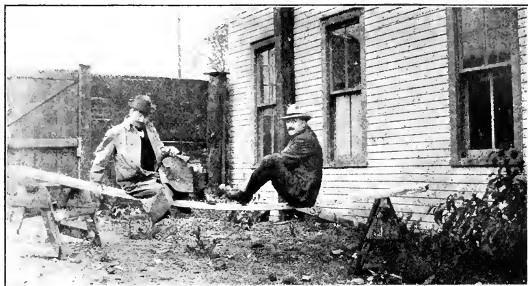
FIG. 13.—DEMONSTRATION OF THE ELASTIC DEFORMATION OF BALSA WOOD.
